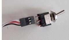
**Toggle Switch** - You can also use a toggle switch to control the SwitchWright by putting on the Tgl Jumper as shown. A SPST (on-off) toggle will do, although if you use a DPDT as illustrated you can use the extra contacts to wire the frog power. Attach the switch across the two Controller end posts (signal and ground) skipping the middle post.
