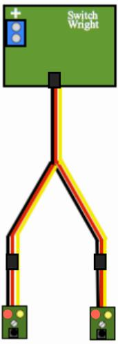
A Y cable can be used to connect 2 Fascia Controllers. Both controllers will act the same.
