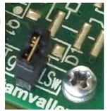
**LSwp Jumper** - this jumper swaps the LEDs on the controller. Use to align the controller with the direction of the points after mounting.
