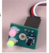
**Install Centering Jumper.** The centering jumper is used to put the servo in the precise center. The jumper is ON when it covers both pins. If it is on one pin or no pins, it is OFF. Center the servo while installing.
