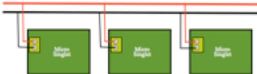
For multiple boards, wire the boards in parallel as in the diagram. Connect the servo and fascia controller as illustrated above.
