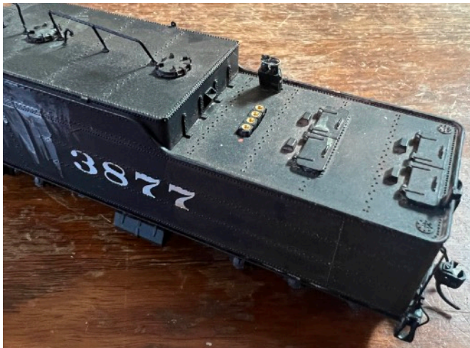
Example installation in BLI steam tender. Power plug is shown in on position
