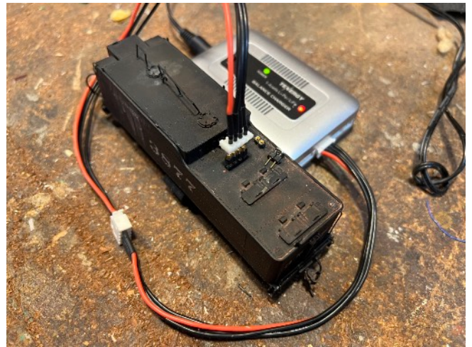
Charging with Tenergy balancing charger. Note that power plug is off. Leaving on will confuse charger and result in overcharging.
